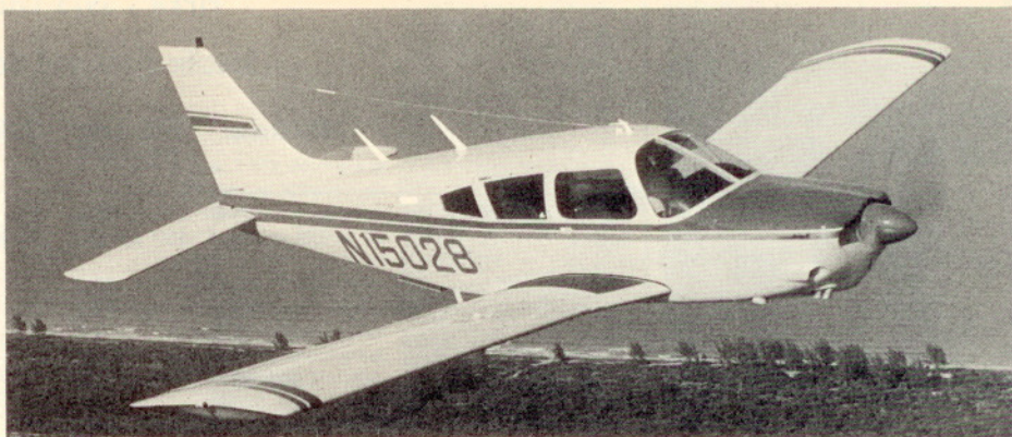
The four-place Cherokee Arrow II, the retractable-gear member of the Cherokee tribe, has a landing gear that automatically extends when speed gets down to 105 mph. New this year is an airspeed sensor that prevents gear retraction on takeoff until climb speed exceeds 85 mph. An override system lock is provided.
